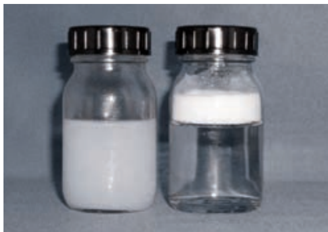
Figure 11: Water with hydrophilic silica (left) and hydrophobic silica (right)
