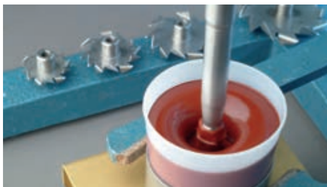
Figure 26: Dispersion with a dissolver
