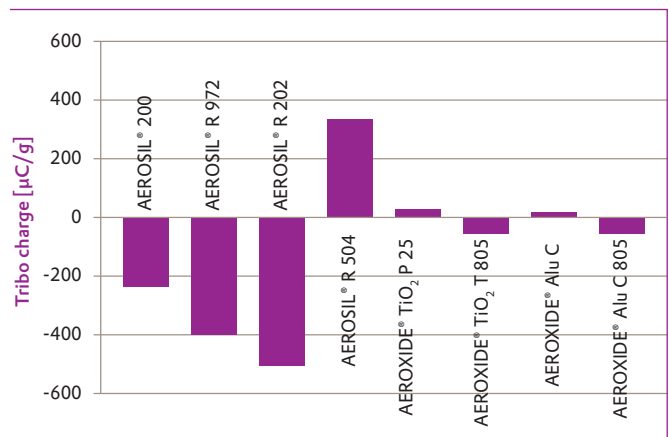
Figure 19 shows the specific charge values (q/m values, charge-mass ratios) for selected products
