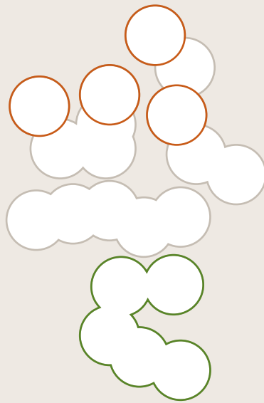
Figure 3: Diagram illustrating the terms primary particle, aggregate, and agglomerate
