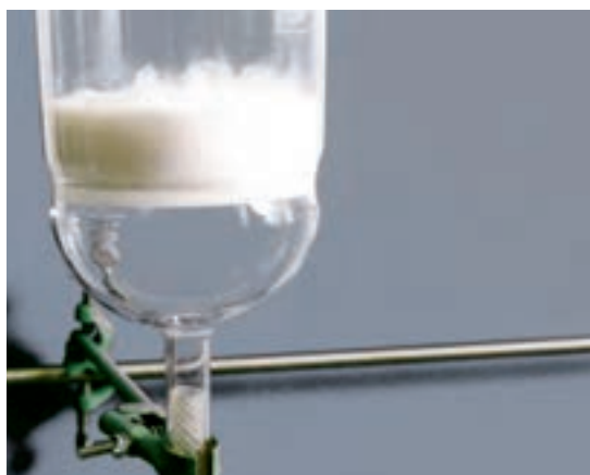
Figure 33: Simple lab demonstration of the fluidization of AEROSIL®. Compressed air with a pressure of approximately 0.2 bar is applied to the glass frit.
