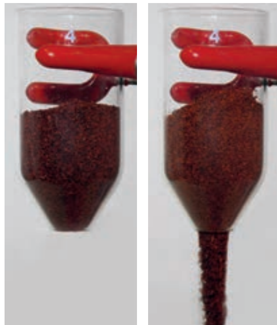
Figure 82: Free-flow properties of chili powder Left with no flow enhancer, right with 2% AEROSIL® 200 F
