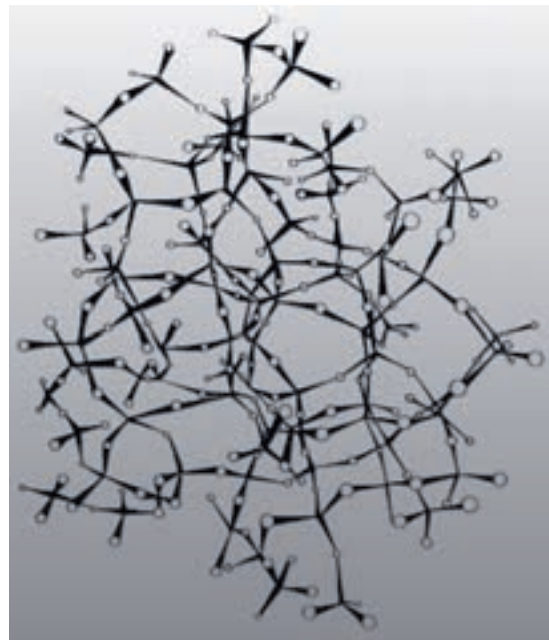
Figure 31: Diagram of the arrangement of SiO 4 tetrahedrons in AEROSIL®, based on a model by EVANS and KING [10]. The circles represent oxygen atoms. The silicon atoms are located in the centers of the tetrahedrons.
