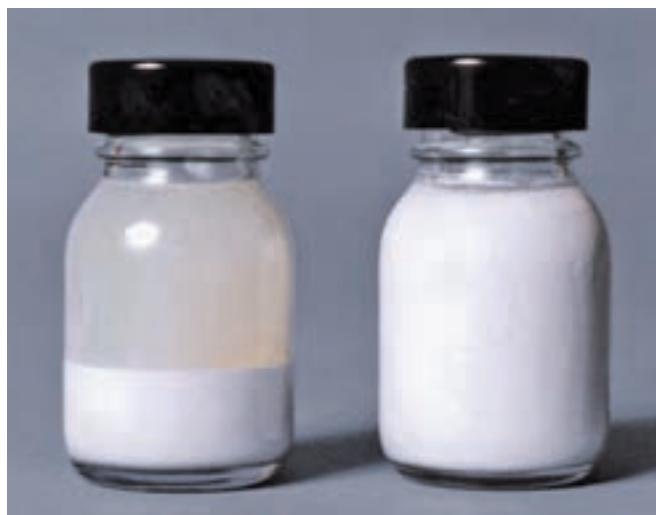
Figure 80: Separation after eight weeks' storage at room temperature Left: No AEROSIL®, right: 0.8% AEROSIL® R 972 Water-based filler based on PUR dispersion/melamine resin
