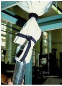
**Figure 19**Removing the PESy from the discharge spout
