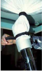
**Figure 10**Fixing the PESy to the discharge spout of the FIBC
