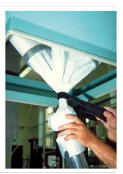
Figure 18 Closing the discharge spout
