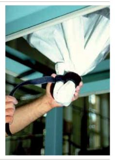
**Figure 20**Tying the gooseneck for dust-proof closure of the FIBC after it has been emptied
