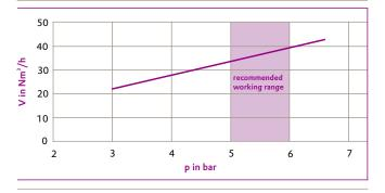
This means that 39 Nm³/h of air at 6 bar is to be provided during the fluidization pulse. However, for example with fluidization of 1 second pulse and 9 seconds pause, the resulting air consumption is just 3.9 Nm³/h. To actually provide this air volume on the PESy during the short pulse, the solenoid valve and the feed hose must not be too small. An inner diameter of 12 mm has proven to be suitable. The distance between the solenoid valve and the PESy should also not exceed 5 meters.
