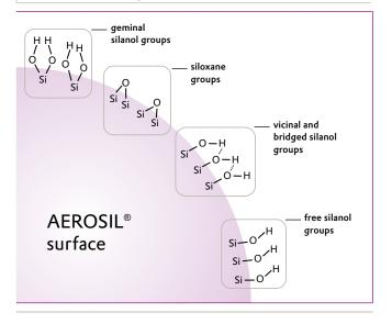
Schematic compilation of different surface-functional groups located on the surface of AEROSIL® products.
