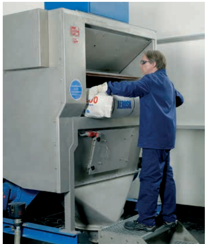
Figure 5 Semi-automatic bag-emptying machine (Manufacturer: Dinnissen B. V, 5975 NB Sevenum, Netherlands)
