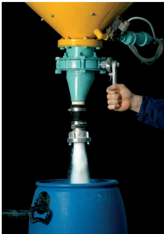
Figure 19 Demonstrating the flow properties of synthetic silica being discharged from a silo containing a fluidizing base as an emptying aid
