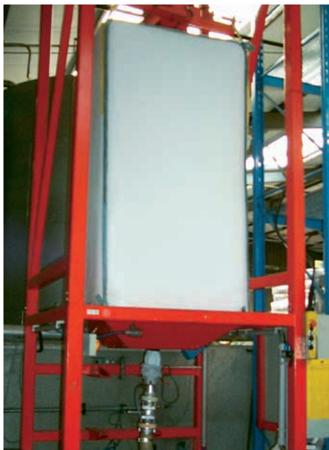
Figure 8 Discharge of precipitated silica from an FIBC
