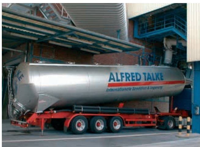
Figure 3 Example of a bulk truck used for AEROSIL® fumed silica and precipitated silica
