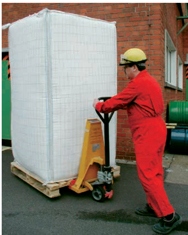
Figure 2 Example of a FIBC (Flexible Intermediate Bulk Container)
