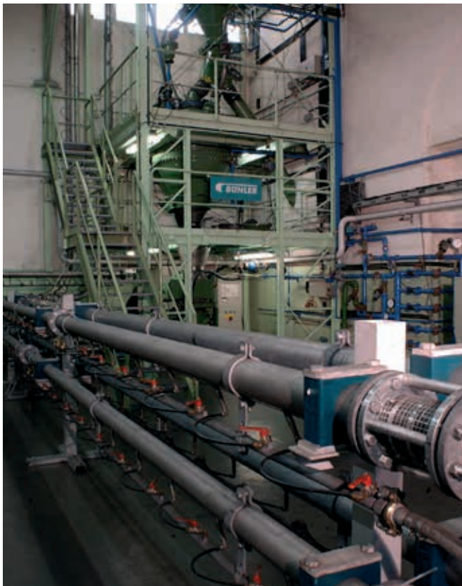
Figure 12 Dense phase conveying system for granulated silica
