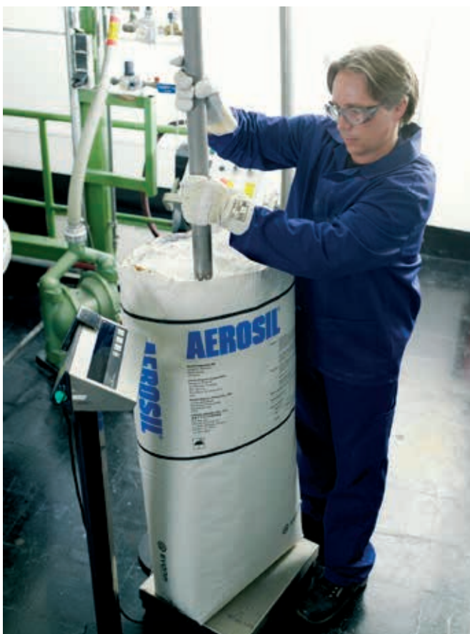
Figure 29 Differential weighing by extracting synthetic silica from a bag by suction
