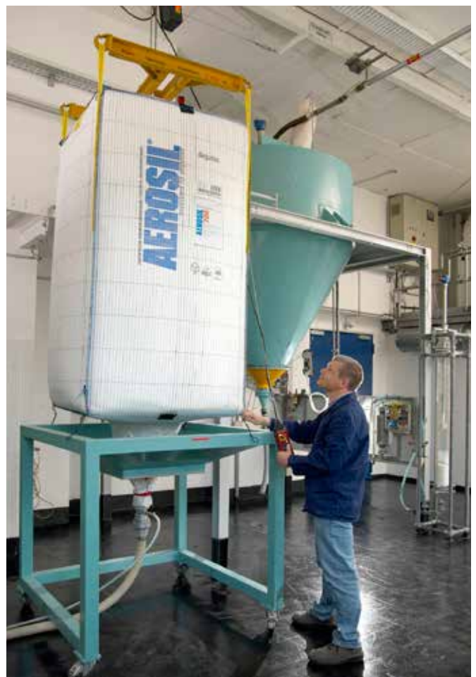
Figure 9 FIBC before discharge
