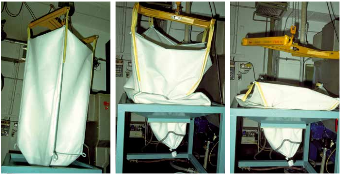
Figure 24 Removing the FIBC from the lifting apparatus
