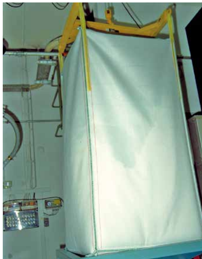
Figure 18 FIBC during discharge
