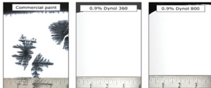
Vinyl acrylic interior commercial paint applied to a contaminated surface crawls and has major film defects. The same paint with 0.9% DYNOL™ 360 surfactant and DYNOL™ 800 surfactant wets the contaminated surface perfectly.
