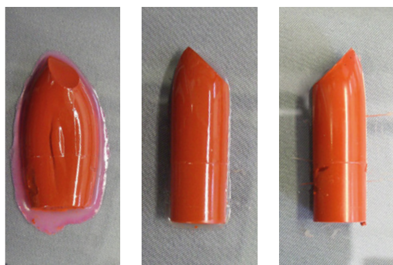
Figure 10: Lipstick after high temperature storage (4 hours at 65 °C) Left: lipstick containing no silica has deformed due to temperature and has sweated out a large portion of oil. Center and right: lipsticks containing 2 % and 4% w / w SIPERNAT® 500 LS (respectively) have retained their shape and oil. Figure 11: Powder to cream lipstick formulation
