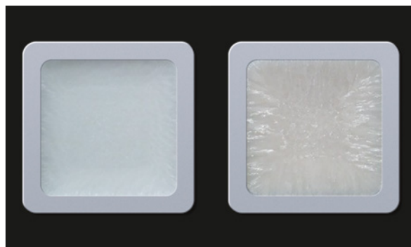
AP Stick with 3.0 wt.-% AEROSIL® R 972 (left), 3.0 wt.-% Bentone 38 V (right). AEROSIL® formulations showed very little whitening compared to sticks containing Bentone (Elementis specialties)
