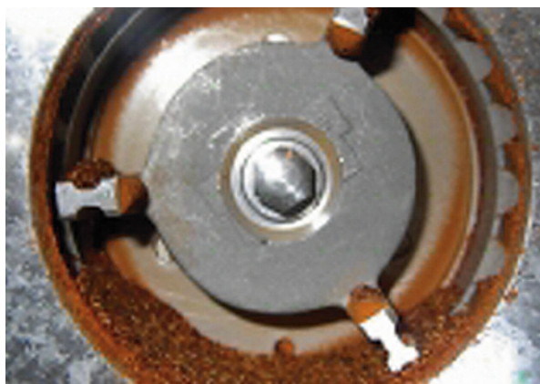
Example: Chili powder in a hammer mill Without milling aid, the powder sticks to the wall and blocks the mill
