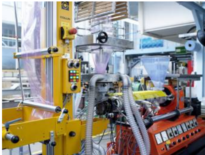
Production of blown film virgin resin + 2 % of the masterbatches
