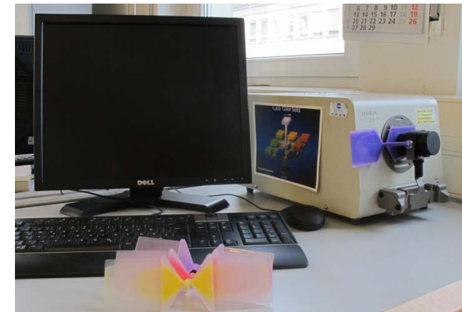
measurement of the color yield, (X,Y,Z values, or L*a*b* values DIN 53 235 )
