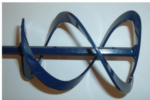
Figure 3: Mixing equipment (cement mixer, l = 14 cm) to homogenize TEGOSOFT® LSE 65 K types (mainly before analytical tests)
