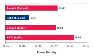
Plastistrength® 566 provides superior inward foaming effect (lab scale simulation of Celuka process)
