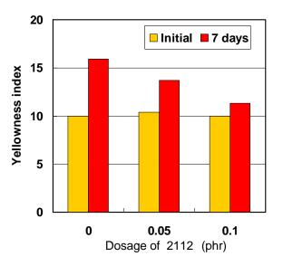
Fig.2 Discoloration in long-term heat stability test
