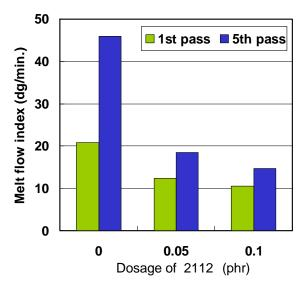
Fig.1 MFR-change (repeated extrusion)
